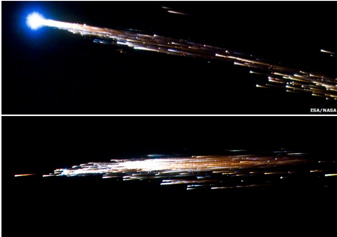
Figure: Early and Late Images of the destructive re-entry of ATV-1 (Courtesy of NASA)
